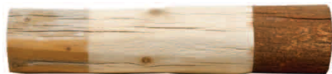
Corn cob media blasting. The bare wood shown in the middle DOES return to its natural color after cob-blasting.
